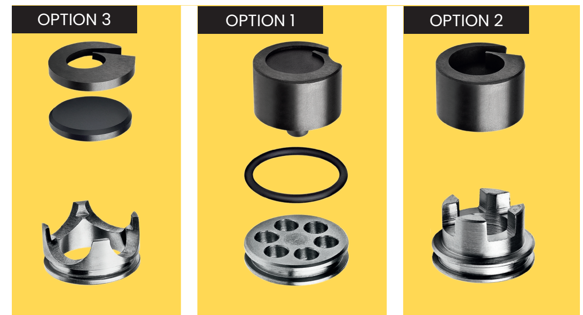
Option 3 The open swirl chamber is ideal for highly abrasive applications since the end plate can be replaced completely independently of the swirl chamber.
