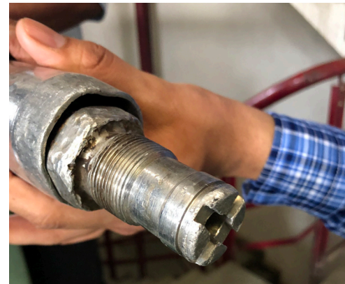
Damage to threads on SDX® III Nozzle.
