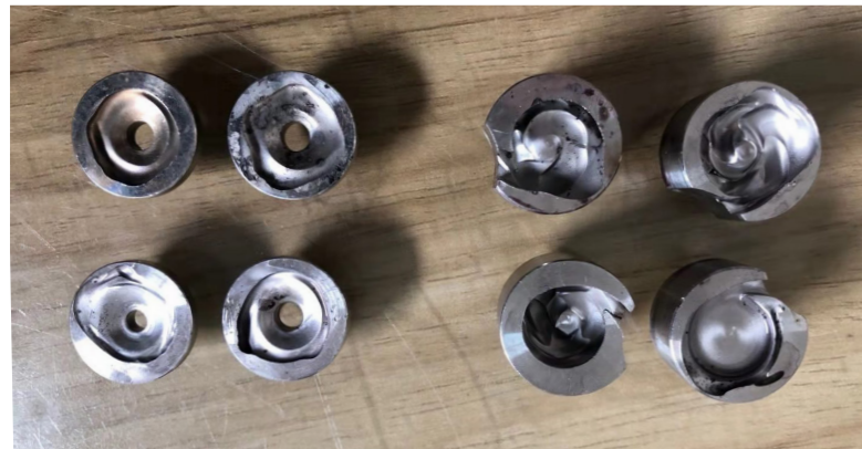
Incorrect orifice and swirl chamber material selection, resulting in premature wear. For advice on material and compatibility contact Delavan®.
