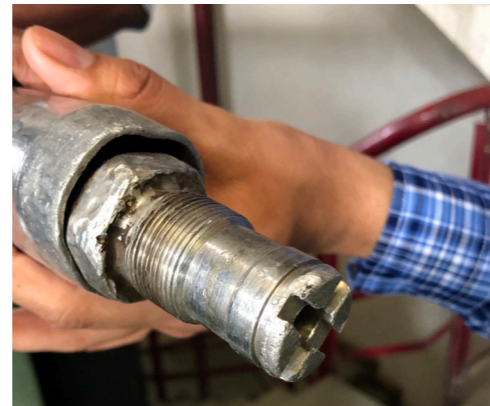
Damage to threads on SDX® III Nozzle.
