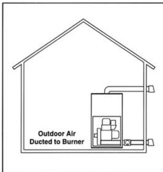
FIGURE 28 Outside air combustion
